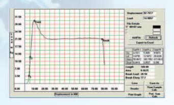
Graphic display and printout through PC: Peak load, Break load, Elongation at peak load, Elongation at break load, Tensile strength at peak load, Tensile strength at break load, % Elongation at break load, Young's modulus, Yield load, Yield stress and Load Vs Elongation graph could be obtained by attaching a printer to the PC. Similarly average value and standard deviation could be obtained by merging different tests.
